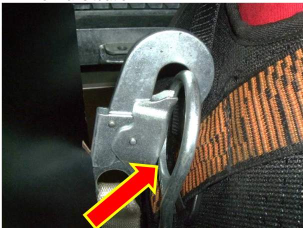
1.4 Lock activated by own back-ring
