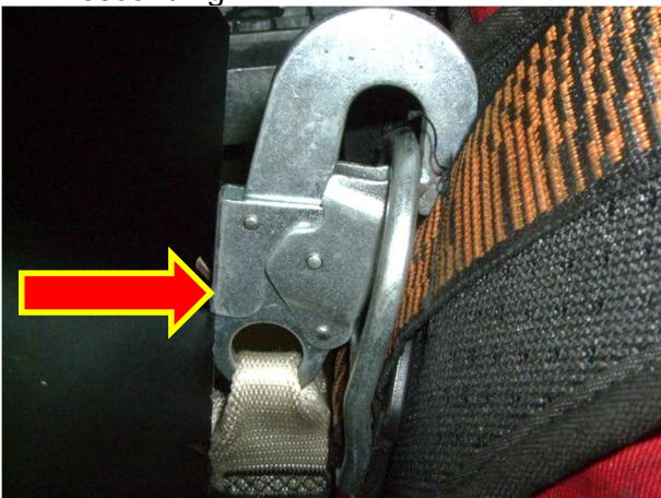
1.3 Safety lock activated by hatch
